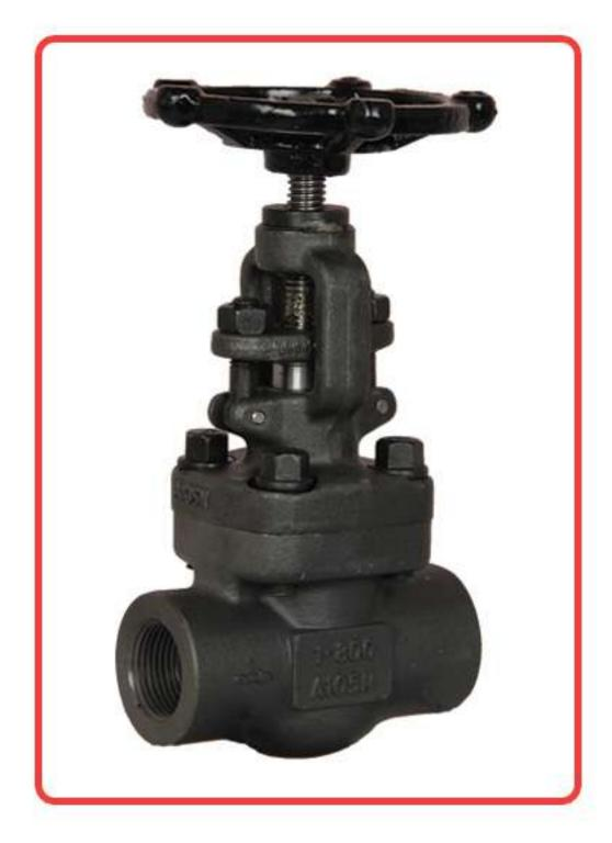
Forged Steel Globe Valves are generally available with Plug Type Disc, which is designed to give leak tight seating over a long period of in built wear life. All Globe Valve stem is made from solid one-piece construction. The yoke bush of Globe Valve has a long thread engagement for accurate stem alignment.
