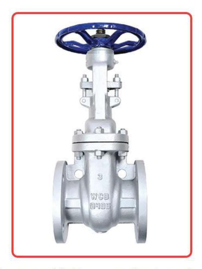
Designed for high pressure and high temperature applications, for a wide range of fluids except slurries and viscous fluids. These Valves are generally used in the wide open or closed position, are not recommended for throttling service because throttling causes disc chattering and vibration which is likely to erode the seating surface and cause leakage. The range comprises Valves for cryogenic services, NACE Specifications (MR-01-75), Position Indicator, Drain plug & Bypass Arrangement.
